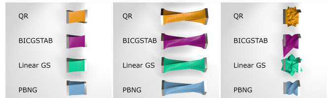
Fig. 11. Hessian Comparison. The top three bars are simulated using Newton’s method with different linear solvers (QR, BICGSTAB and linear Gauss-Seidel respectively). The bottom bar is simulated using PBNG. The top bar uses the exact Hessian and becomes unstable. The bottom bar uses our Hessian projection and stays stable.
