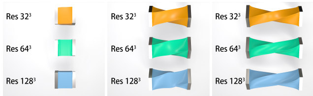
Fig. 8. Different Mesh Resolution. PBNG produces consistent results when the mesh is spatially refined. The highest resolution mesh in this comparison has over 2M vertices and only requires 40 iterations to produce visually plausible results.
