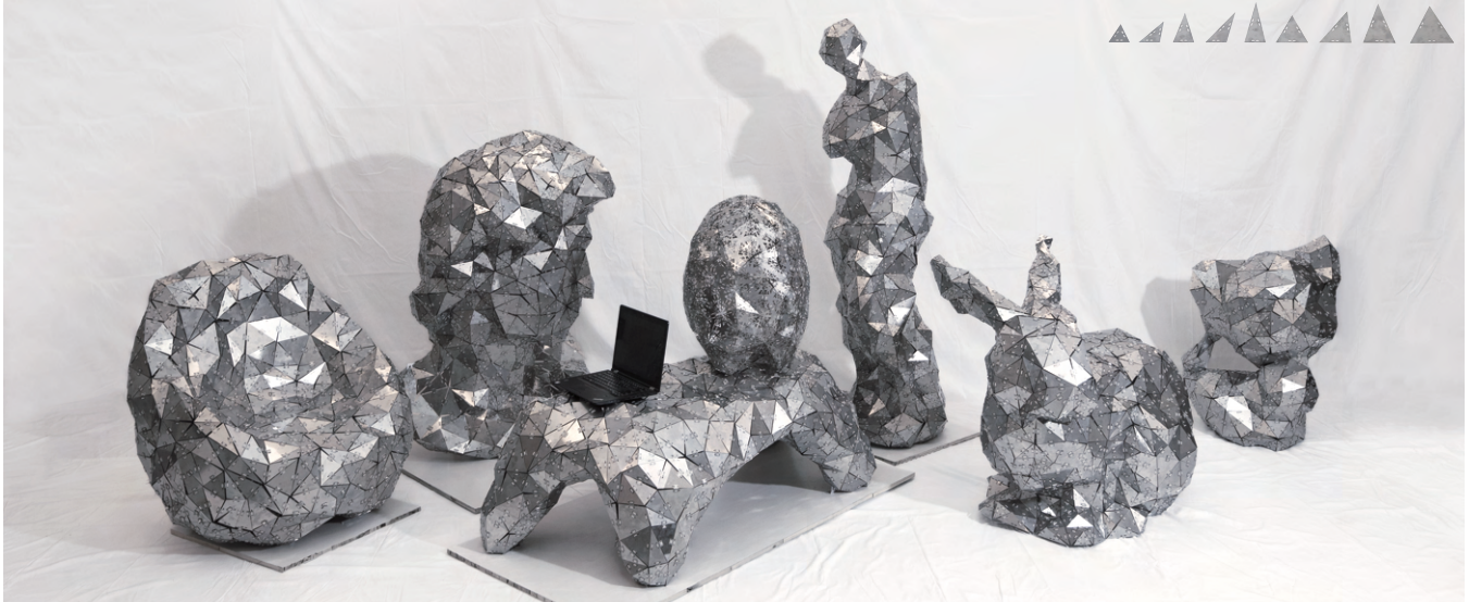
Fig. 1. By applying our method, seven models are modeled and fabricated using nine specified discrete equivalence classes of triangles (shown in the top right corner). They are a modern chair, the David's head, a table, a decorative lampshade, the Venus, the bunny, and the kitten model (from left to right). A real black 14-inch laptop is put on the table as a size reference.
