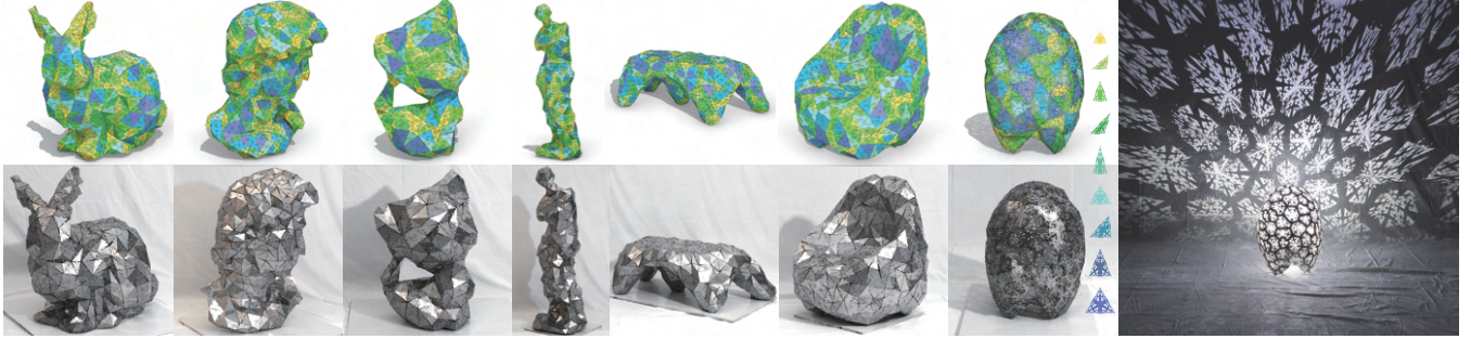
Fig. 18. Gallery of our digital results (top) and real fabrications (bottom) for seven models. The lampshade uses the templates with a specially designed hollow structure. The actual lighting effect is shown on the far right.
